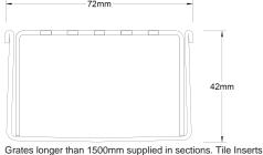
longer than 1200mm supplied in sections. Channels over 3000mm supplied in sections with joiner. +/-2mm tolerance on dimensions.
