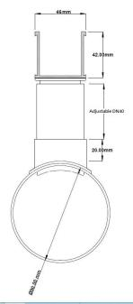
Grates longer than 1500mm supplied in sections. Tile Inserts longer than 1200mm supplied in sections. Channels over 3000mm supplied in sections with joiner. +/-2mm tolerance on dimensions
