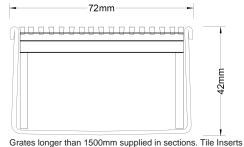
Grates longer than 1500mm supplied in sections. The inserts longer than 1200mm supplied in sections. Channels over 3000mm supplied in sections with joiner. +/-2mm tolerance on dimensions.
