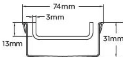
Grates longer than 1500mm supplied in sections. Tile Inserts longer than 1200mm supplied in sections. Channels over 3000mm supplied in sections with joiner. +/-2mm tolerance on dimensions.
