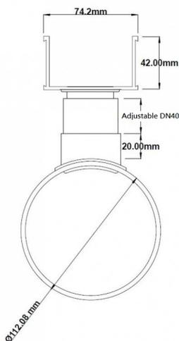
Grates longer than 1500mm supplied in sections. Tile Inserts longer than 1200mm supplied in sections. Channels over 3000mm supplied in sections with joiner. +/-2mm tolerance on dimensions.
