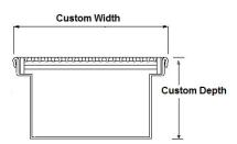
Grates longer than 1500mm supplied in sections. Tile Inserts longer than 1200mm supplied in sections. Channels over 3000mm supplied in sections with joiner. +/-2mm tolerance on dimensions.
