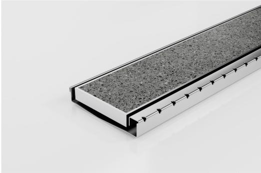
The Shower Screen Support Grate & Channel including 120mm wide Ti grate, with a 16mm screen support bar made from 316 Stainless Steel. Suits tiles up to 10mm thick
